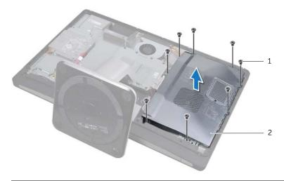
2 screws (8) system-board shield
