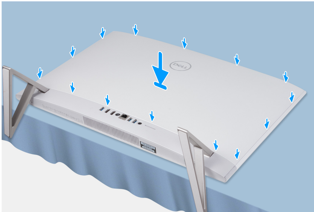
Figure 21. Installing the back cover
