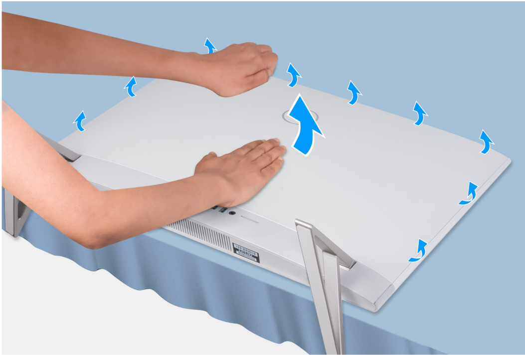
Figure 20. Removing back cover
