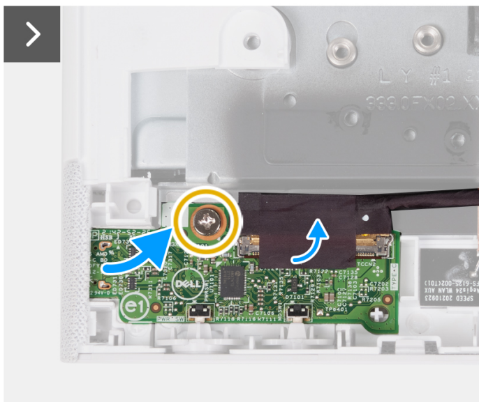
Figure 48. Removing the power-button board with USB
