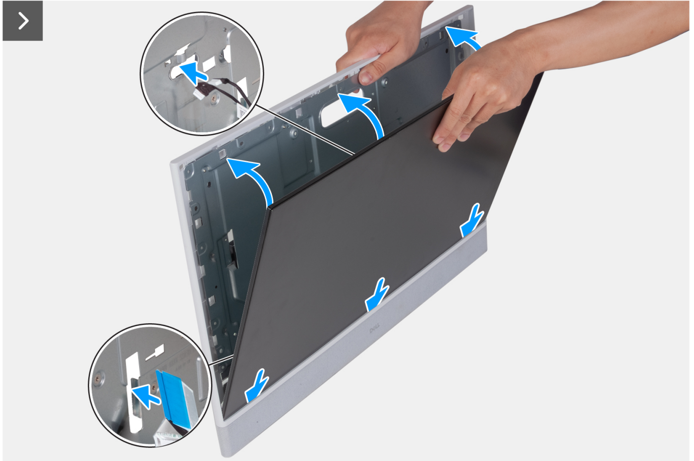
Figure 62. Installing the display panel
