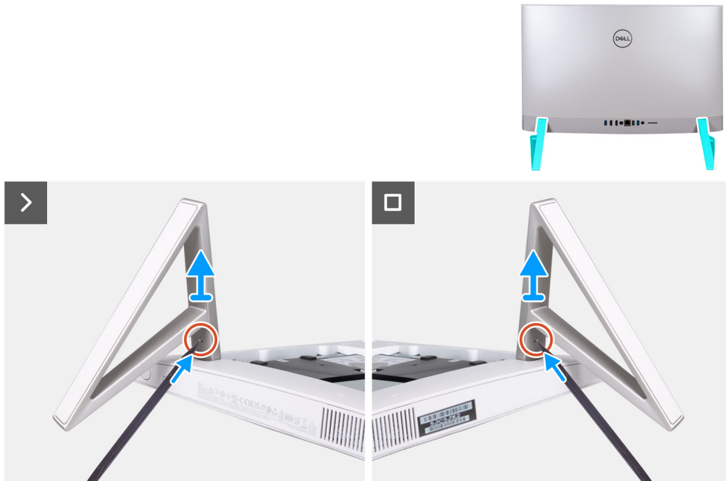
Figure 17. Removing the stand
