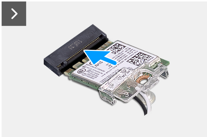
Figure 33. Installing the wireless card
