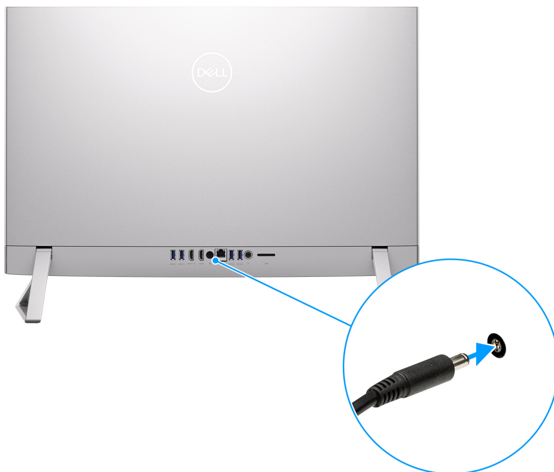
Figure 11. Connect the power adapter .
