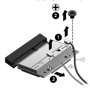
NOTE: If the WLAN antenna cables are not connected to the terminals on the WLAN module, the protective sleeves must be installed on the antenna connectors, as shown in the following illustration.
