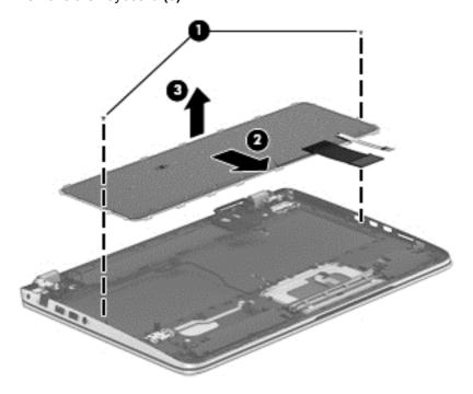
Reverse this procedure to install the keyboard.
