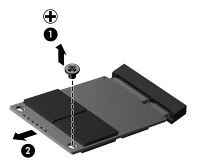
Reverse this procedure to install the mSATA SSD.
