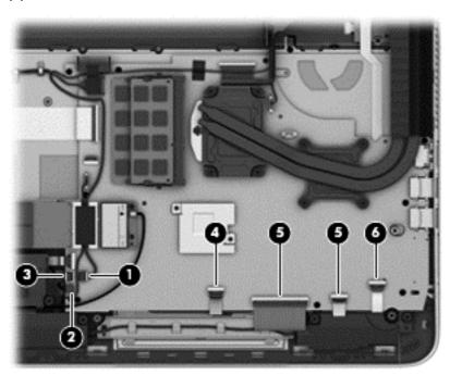
3. Remove the nine Phillips PM2.0×2.9 screws that secure the system board to the top cover.
