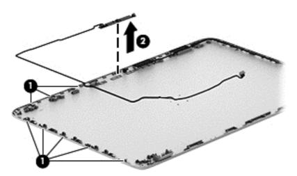
**c.** Remove the webcam/microphone module.
