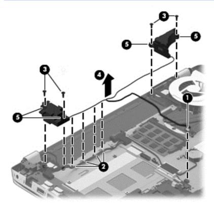
Reverse this procedure to install the rear speakers.
