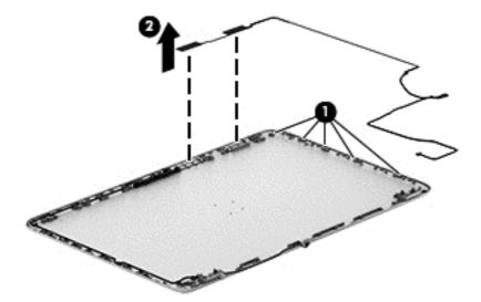
**c.** Remove the wireless antenna.
