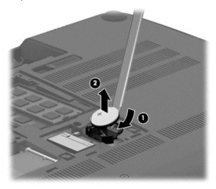
Reverse this procedure to install the RTC battery. When installing the disc cell RTC battery, make sure the "+" sign faces up.
