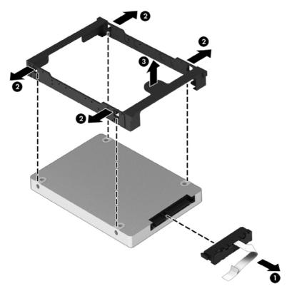
Reverse this procedure to install the hard drive.
