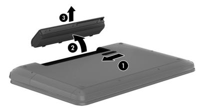
Reverse this procedure to install the battery.
