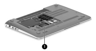
2. Remove the Phillips PM2.0×2.5 screw (1) that secures the mSATA SSD to the system board. (The drive tilts up.)
