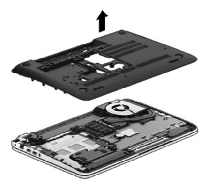
Reverse this procedure to install the base enclosure.
