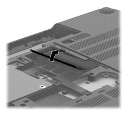
2. Spread the retaining tabs (1) on each side of the memory module slot to release the memory module. (The memory module tilts up.)
