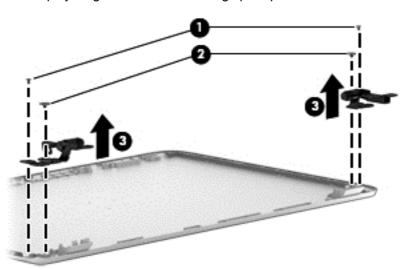
**c.** Remove the three Phillips PM2.0×2.9 screws **(1)** that secure the left and right display hinge brackets to the display enclosure.
