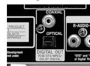
Coaxial and optical digital audio outputs
