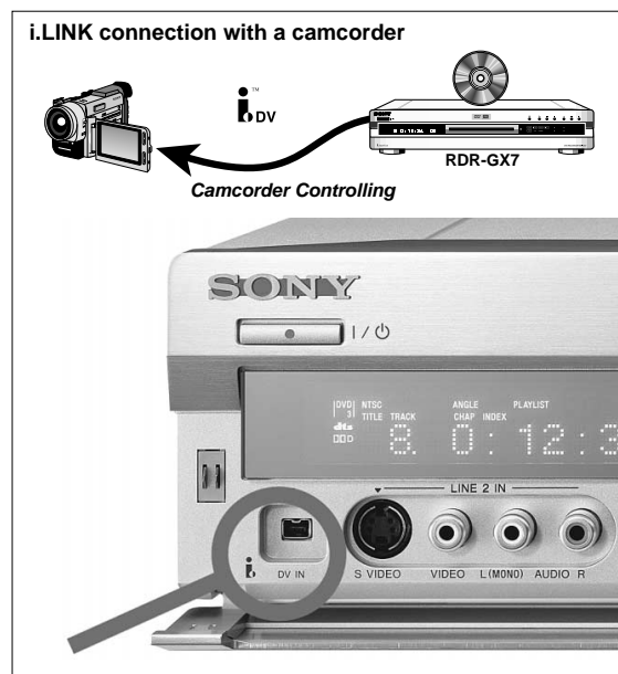
An i.LINK (DV) IN terminal is provided on the front panel.
