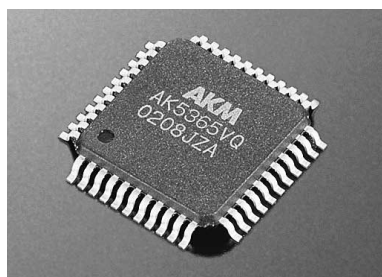
The Newly Developed 96 kHz 24-bit Capable A/D Converter
