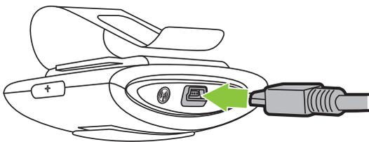
The main indicator light turns red or yellow when the battery is charging. It may take up to 1 minute for the indicator light to turn on. When the T505's battery is close to fully charged (about 5 hours), the indicator light turns green.
